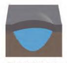
COLD FREEZES THE WATER, CAUSING IT TO EXPAND & FORM A BUMP IN THE ROAD.
