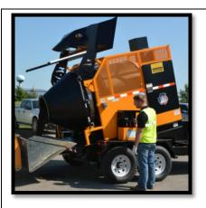
16. RAISE DRUM. Use the hydraulic dump lever to raise the drum approximately twenty (20) degrees. Continue rotation until the drum has been emptied. The flights inside the drum will assist in the dumping of the asphalt material. The flights will push the RAP to the drum opening. It is not necessary to raise the drum to its full up position to empty the drum. The drum should be raised to a position that causes the RAP to dump cleanly and easily.
