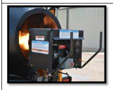
11. START BURNER. Turn the toggle switch ON. The Burner has a 5 second pre-purge delay before fuel introduction and ignition. The pressure gage should be steady at 120 psi. The burner nozzle may drip some fuel into the drum while it is warming up.
