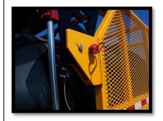
4. CHUTE PINS. When the loading chute is in the up and pinned position the safety Locking Pins must be removed prior to moving the loading chute into the down or loading position.
