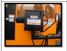
8. MOVE BURNER. Remove the burner from its travel position. This will require the removal of the safety pin; the spring loaded locking pin and the "T" handle, threaded position lock and the pinned travel cover. The pinned travel cover is located on the front of the burner.
