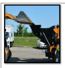
6. LOAD MATERIAL. Load asphalt material into the rotating drum through the loading chute until the drum is full. NOTE: the drum is full when it will not accept any additional material without excess spillage from the drum opening.
