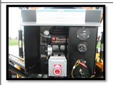
10. POWER BURNER. Turn the red 12 volt power key to the on position (Figure 3). Verify a minimum of 12 Volts is supplied at the burner.
