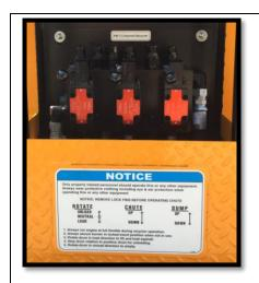
1. HYDRAULIC CONTROL VALVES. The Hydraulic Control Valves, located on the rear passenger side fender, must all be in the neutral position prior to starting the engine.
