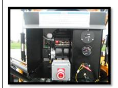
14. SWITCH OFF BURNER. Turn Toggle switch to the OFF position and allow the Burner to complete its' fifteen (15) second (previously 30) post purge cycle. Turn Red 12 Volt Power Key to the OFF position. Remove the Burner Arm Lock Pin and return the Burner to its travel position: lock the arm in place to avoid physical damage while dumping the load.
