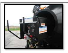
9. POSITION BURNER. Move the Beckett Burner into position inside the drum opening. Place the Burner locking pin in place (Located at the base of the arm by the fender,) and tighten the "T" handle position lock.
