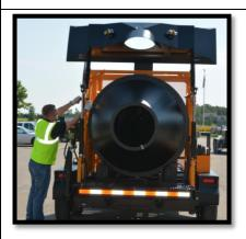
7. CHUTE UP. Move the loading chute to the "UP" position and replace safety Locking Pins.
