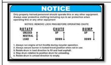
15. REVERSE DRUM TO UNLOAD. Move the drum rotation hydraulic selector lever to the NEUTRAL position to stop the drum rotation. REVERSE DRUM. Move the drum rotation lever to the unload position to reverse drum rotation and begin emptying the drum.
