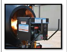
13. HEAT TIME. Heating times will vary due to outside temperatures, the type and quality of recycled asphalt material (RAP), which can vary dramatically from area to area, and RAP moisture content. The KMI supplied Infrared Thermometer should be used during heating to check asphalt temperature. Optimum temperature of the entire mix should be 335 degrees Fahrenheit. Optimum temperature should be reached prior to dumping. If temperatures vary the lowest temperature should be used.
