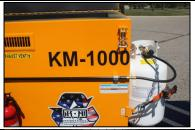
**1**. Slowly open the propane cylinder. Be sure not to activate the safety excess flow valves in the bottle fittings.
