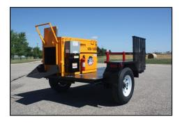
The KM 1000 is fitted with a shovel tray that bolts directly to the shovel door tracks. Use 3/8" locking nuts to fasten the shovel tray.
