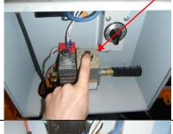
**5**. Push the control knob all the way in and hold. Immediately push the electric igniter button. Continue to hold the control knob while visually checking to see that the pilot light has lit inside the heating chamber along the burner.
