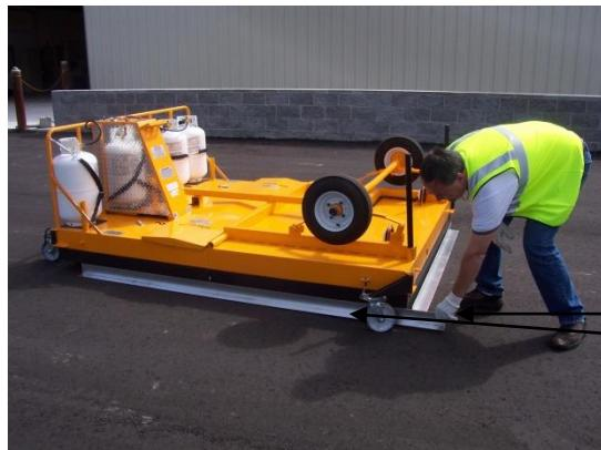
**⚠️ WARNING:** Gloves MUST be worn when adjusting or removing wind skirts. The skirts are made of aluminum and quickly become **very** hot during operation. Handling without proper safety gloves may cause injury.
