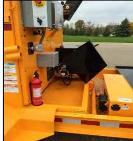
Burner and other key components are located above trailer frame and in steel enclosure. By locating the burner above the trailer frame it is protected from road debris and grime, resulting in a low overall maintenance cost.
