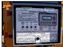
Diesel control panel utilizes PLC and HMI digital control system. Control panel has 168 hour (7 day) on delay timer and low temp thermostat.
